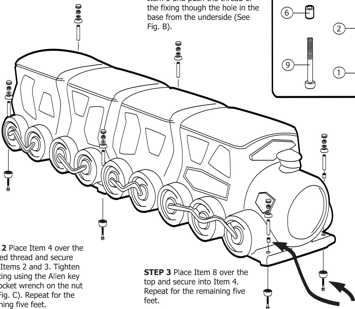
**STEP 2** Place Item 4 over the exposed thread and secure using Items 2 and 3. Tighten the fixing using the Allen key and socket wrench on the nut (See Fig. C). Repeat for the remaining five feet.
